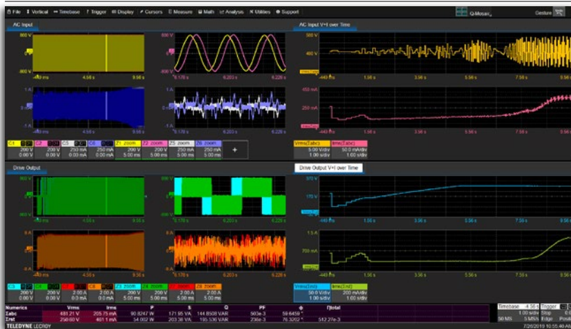
Capture voltage, current and other signals and calculate dynamic responses using per-cycle Waveforms to better understand complex drive, control and motor behaviors.
